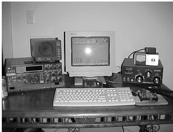
The K2AXX 1999 ARRL Contest Location. See – it really isn't very much of a station. CT keys the radio, have a paddle just in case I need to fill info not in the keyboard buffer.
